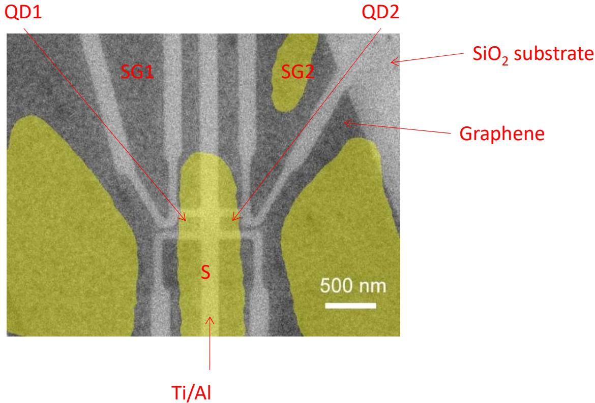
Physical separate two QDS: 1) bias can be tuned independently.
